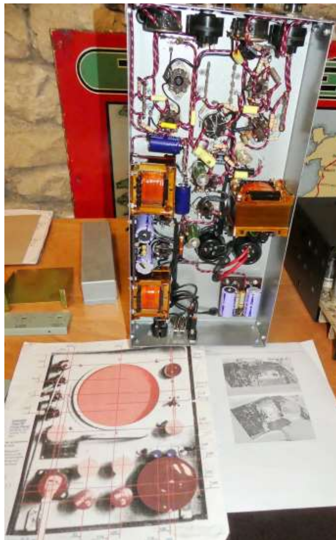
Above , close-up of Tony Waller's early airborne GEE; below , detail of the underside wiring
