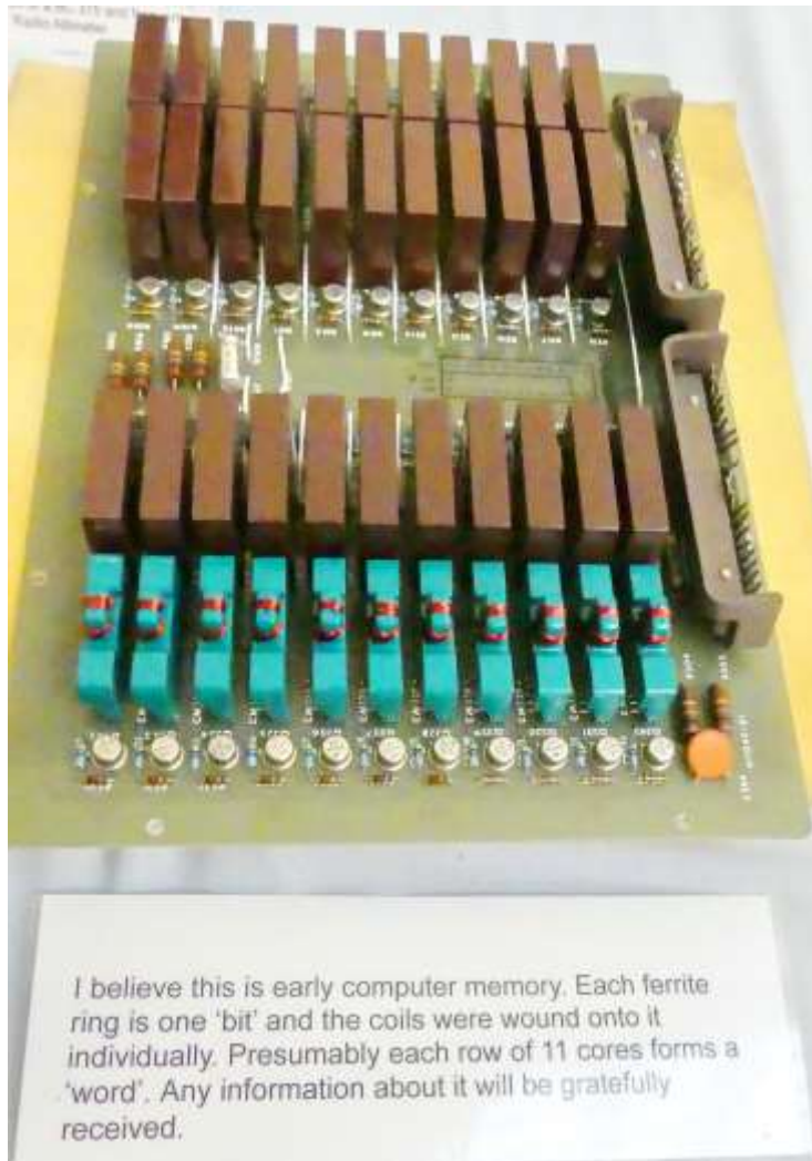
Illustrating the span of DEHS interests, above , early computer ferrite ring memory; below , wet cells.
