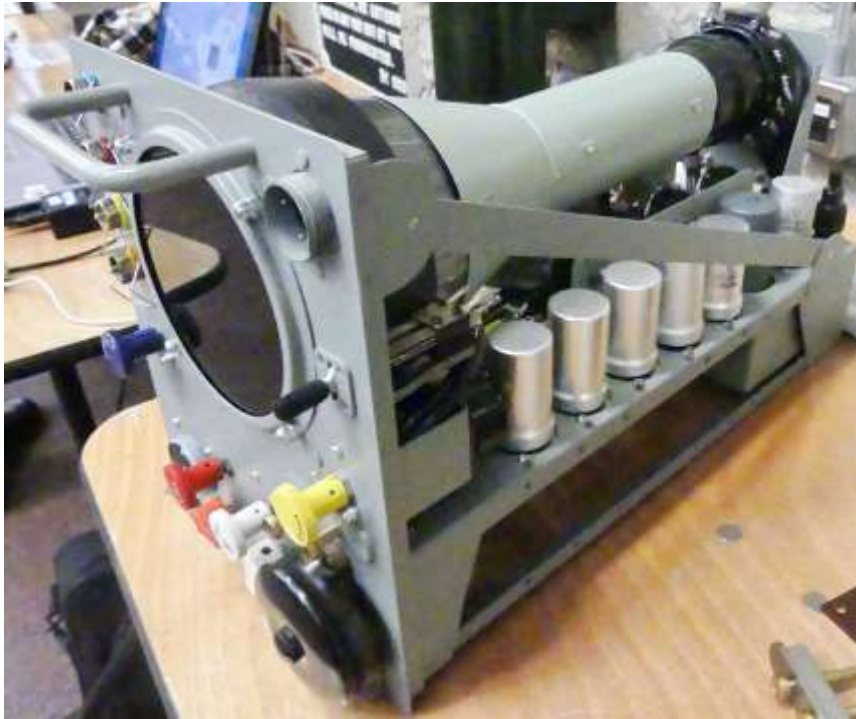
Above , close-up of Tony Waller's early airborne GEE; below , detail of the underside wiring
