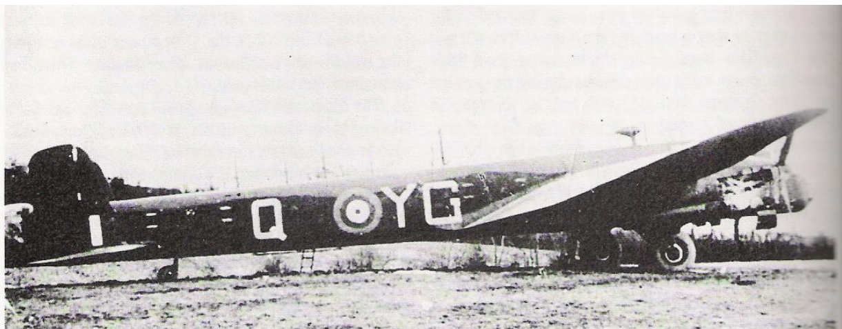
The first unit operational with ASV radar was No.502 Squadron. The extra aerials can be seen mounted on the top of the fuselage of Whitley V, YG-Q, at Limavady early in 1941. (via A.S. Thomas)
